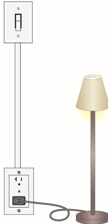
Where a switch controls a receptacle load
